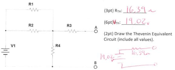
6. (12pt Nodal Analysis) Solve the circuit below using Nodal Analysis. The Reference node and the 3 nodes to solve for have already been placed for you.
