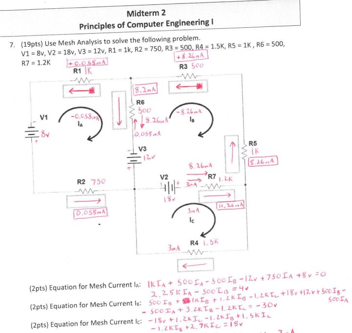
(6pts) Mesh Current IA: 0,058 MA Mesh Current IB: - 8, 26 MA Mesh Current Ic: 3mA
