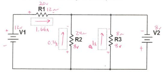
$R_1 = 12\Omega, R_2 = 24\Omega, R_3 = 8\Omega, V_1 = 12v, V_2 = 8v$
