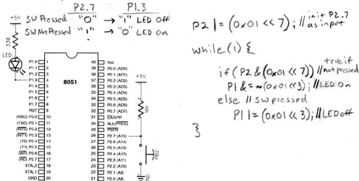
Write a piece of code that infinitely loops and checks the state of the Push Button on P2.7 then turns the LED OFF or ON. When the Push Button gets pushed (i.e. closed) the LED will be turned OFF and when the Push Button is not pushed (i.e. open) the LED will be turned ON. The value written to the port must not change the state of any other pins. Include all necessary C code.
